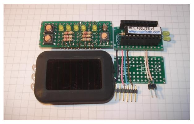
On the left, the 3 LEDs of the Torch, the Solar Cell Cables: Serial / Power Supply 2 Program Pins
